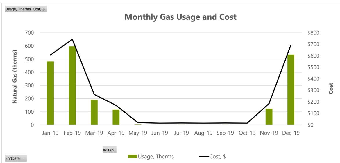
The gas is broken out by end-use in the figure below. Currently, all gas usage is due to the operation of the furnace section of the RTUs during the heating season. There normally would be year-round usage by the water heater, but as observed on site, the water heater isn't currently firing.
